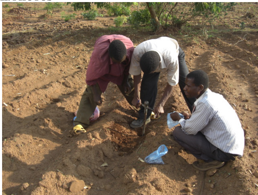
Photo 1: Laboratory technicians from the Department of Agricultural Research Services collecting soil samples from the farmer's field
